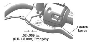
Verify that the safety switch activates properly. The engine should not start in gear with the clutch lever released.
